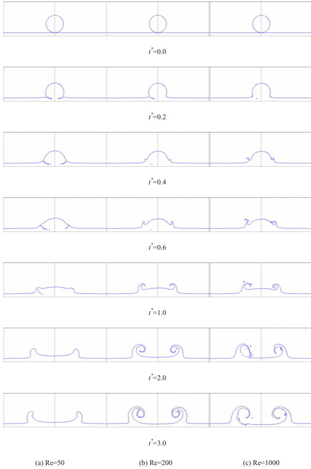
FIG. 12. (Color online) Droplet splashing on a wet surface. Left: Re=50; middle: Re=200; right: Re=1000. In each column, the left frames represent the kinetic-based LBM and the frames on the right are for the phase-field model.
